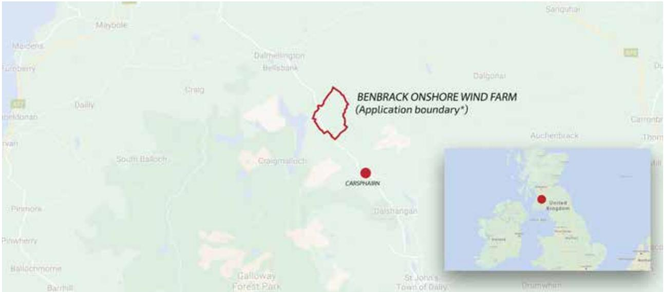
The wind farm site is located just south of the East Ayrshire and Dumfries & Galloway border, approximately 6km north of Carsphairn and east of the A713. Benbrack was first proposed in 2012 and secured planning consent in 2017 which has since been varied to further optimise the project. The wind farm will consist of 15 turbines which have a maximum tip height of 149m and a total generation capacity of 67MW, however there is scope within the consents to potentially increase this.
